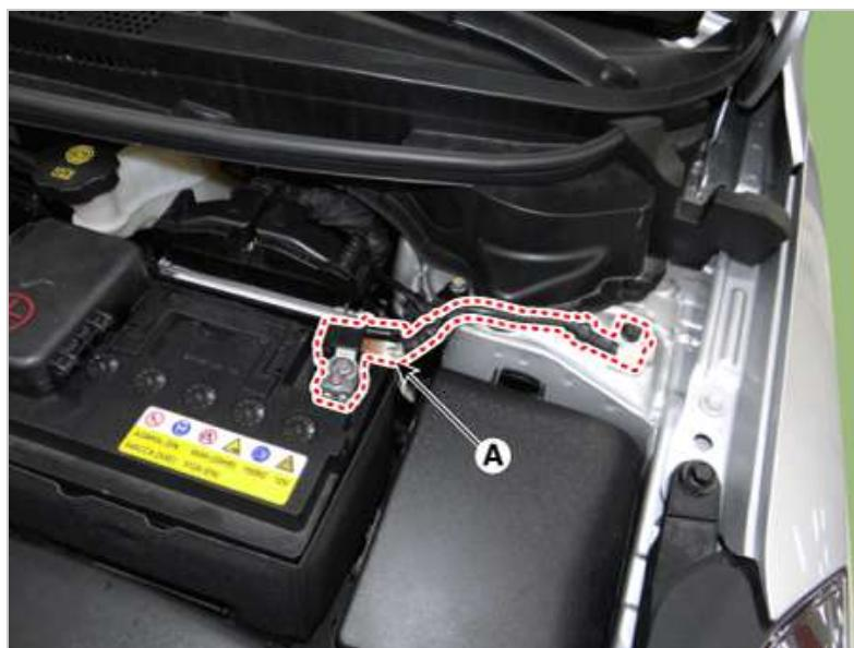
3. Disconnect the positive (+) battery terminal (A).
