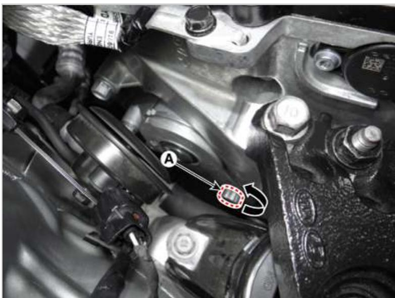
5. Remove the alternator upper mounting bolt (A).
