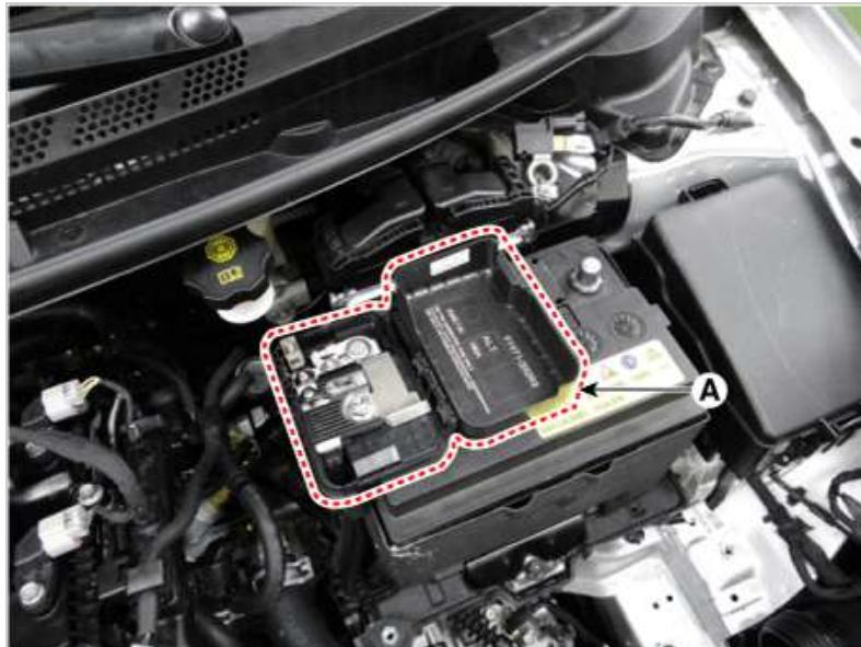
If the battery positive connection is loose, disconnect the ground (GND) cable first before attempting to remove or tighten the positive connection to prevent personal injury.
