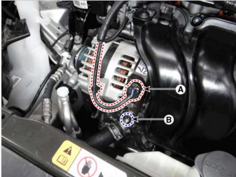
4. Using the hexagon wrench, turn the tensioner (A) counterclockwise and loosen.
