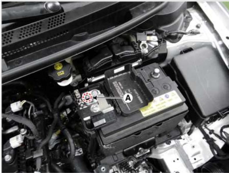
3. If the battery clamp on negative (-) battery terminal is not seated securely:
