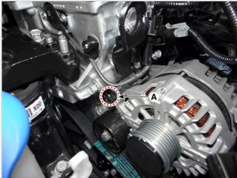
6. Remove the alternator mounting bracket (A) after loosening the lower mounting bolts (B).
